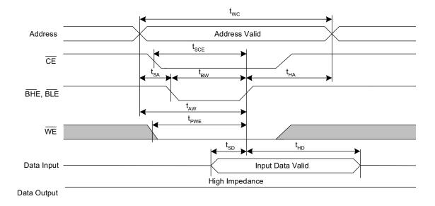
21. Only  $\overline{\text{CE}}$  and  $\overline{\text{WE}}$  controlled writes to RTC registers are allowed.  $\overline{\text{BLE}}$  pin must be held LOW before  $\overline{\text{CE}}$  or  $\overline{\text{WE}}$  pin goes LOW for writes to RTC register.
